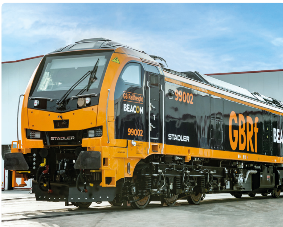
An example of the new hybrid Class 99 freight locomotives now operating on the UK rail network © Stadler Rail.
